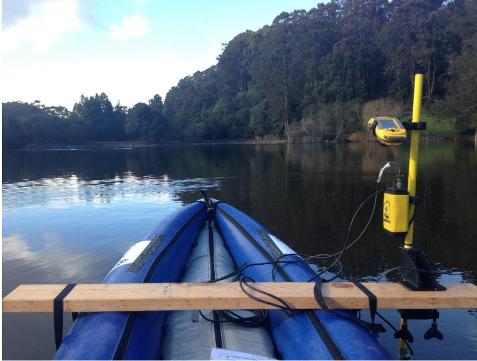
Figure 6: Single beam echosounder and GPS mounted on inflatable kayak for the bathymetry survey of Jewel Lake and Lake Anza.
